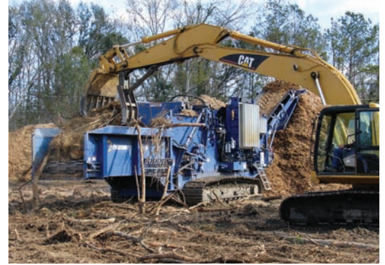
Processing storm debris is another application for the Peterson model 6710B horizontal grinder. Here it's shown in Louisiana after Hurricane Katrina.
