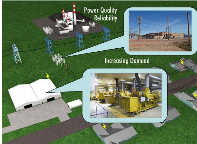
Figure 1: Small scale distributed generation is sited by electric utilities at the substation level or at the point of end use.
