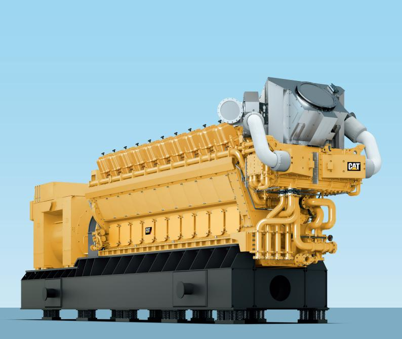
GENSET 4-stroke natural gas engine SPECIFICATION with 20 cylinders and an efficiency up to 48.9 % at a total power output of 10,300 kWe
