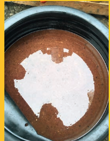
Fuel polishing removed these impurities and sediment from a Peterson customer's diesel tank
